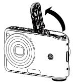
2. Insert the battery while observing the correct polarity. Use the side of battery to press down the stopper as shown, allowing the battery to be inserted properly.
